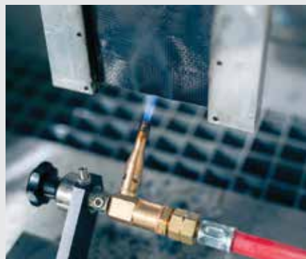
Wall Tight FR G A2 flame-retardant membrane ... extensive testing has proved it to be non-combustible.
